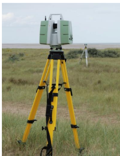
Plate 2: Terrestrial laser scanner
